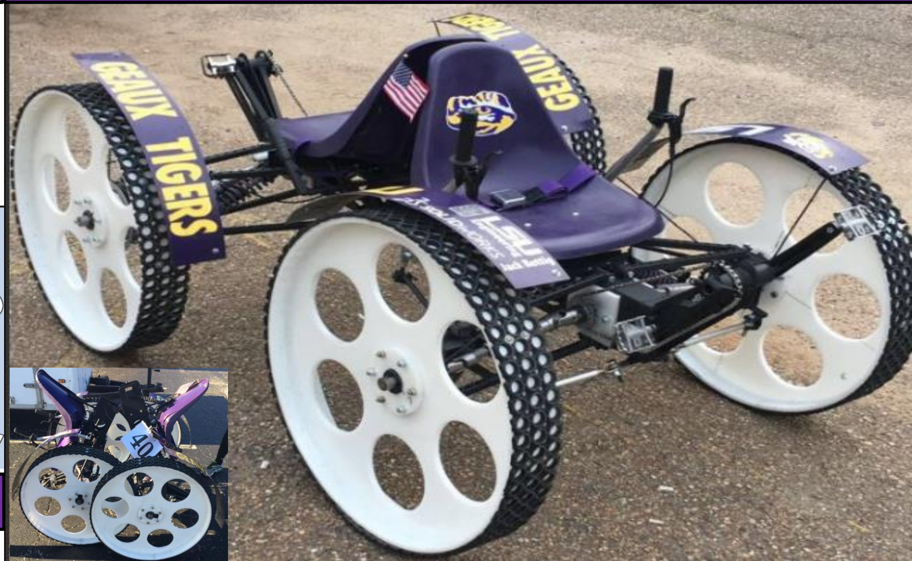
Discs were cut and CNC'd out of HDPE. Channels were milled through the center of the rims and they were put through the roller to bend them into semicircles. A heat gun was used to plastic weld the rims to the disks. Bar mat was secured to HDPE rims with screws and washers
