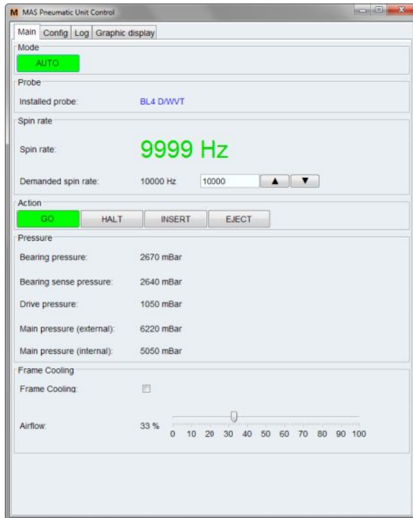
Figure 3.17: MAS II Pneumatic Unit Control Display.
